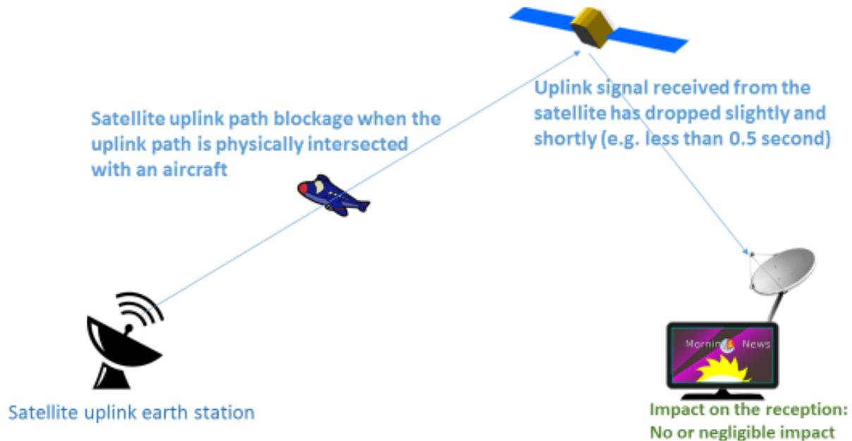
**Figure 7: Situation when satellite uplink path is physically intersected with an aircraft**
