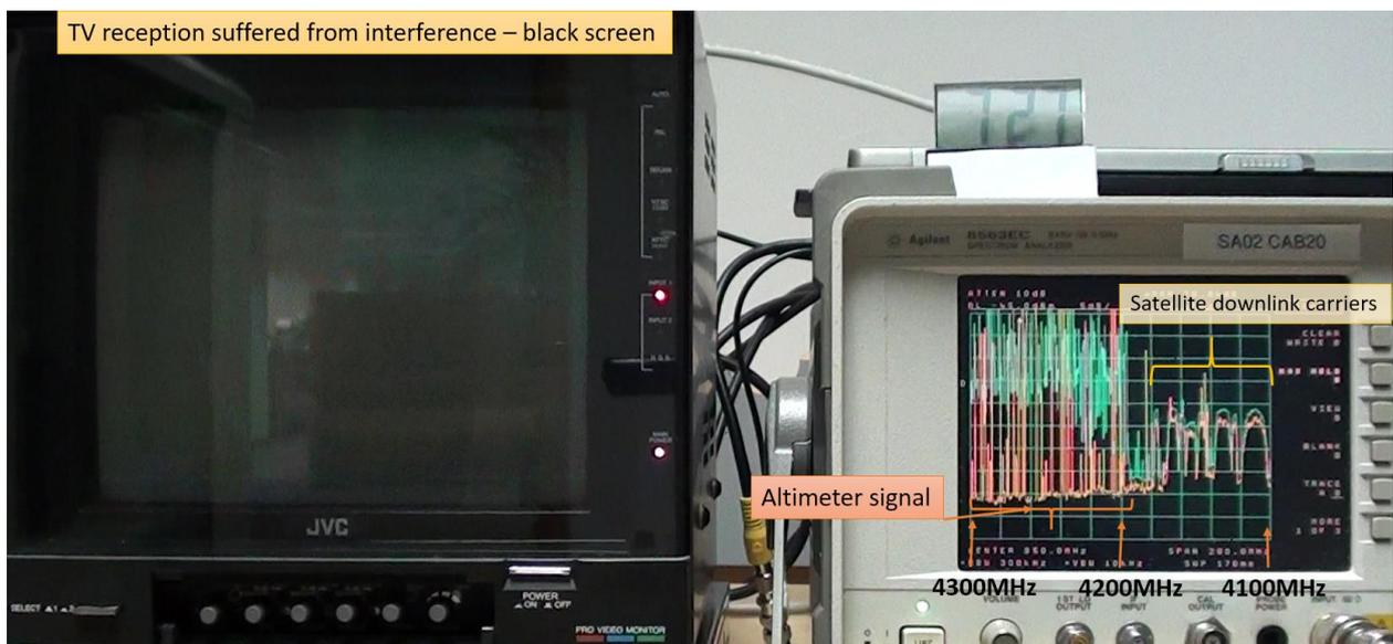
Figure 6: Spectrum plot where a C-band receiver is affected by aircraft altimeter – TV reception: black screen
