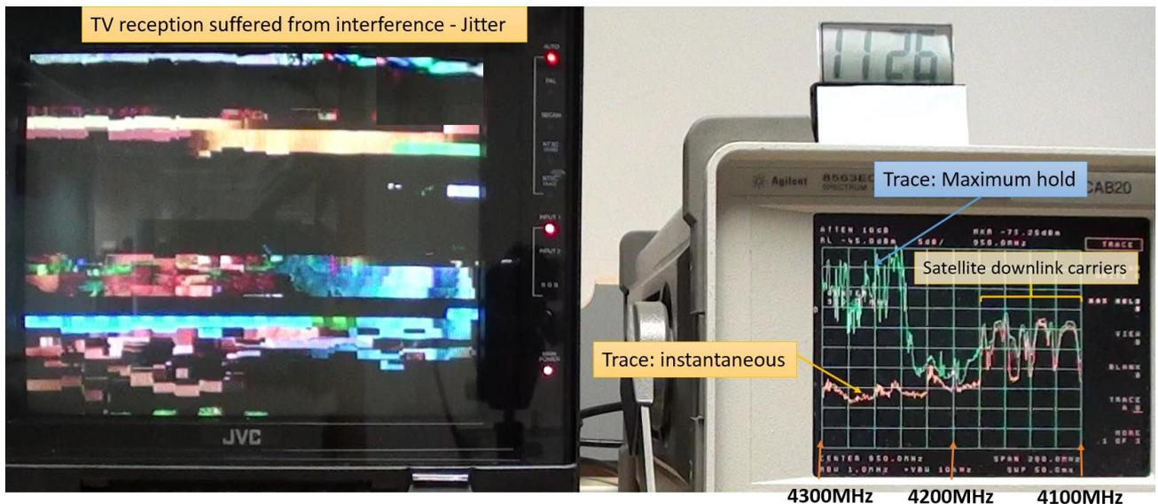
Figure 5: Spectrum plot where a C-band receiver is affected by aircraft altimeter - TV reception: jitter
