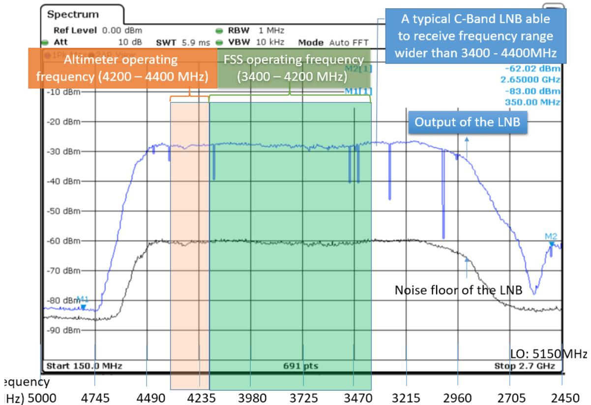
Figure 3: Frequency response of a typical C-band satellite receiver
